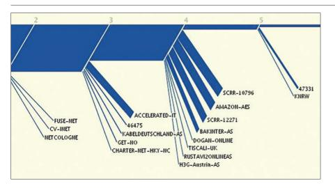
A generated graphic showing BGP hops and traffic volume to various connections.
